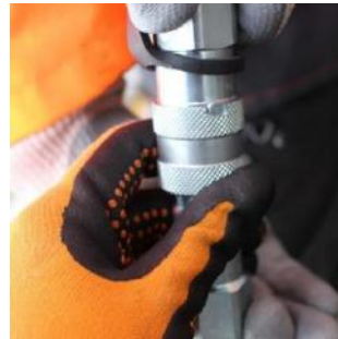
Hydraulic Connection to Flow of Hydraulic Unit
